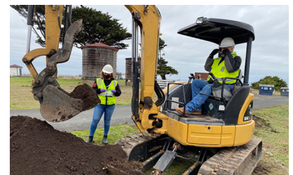
County PID testing of excavated soil
